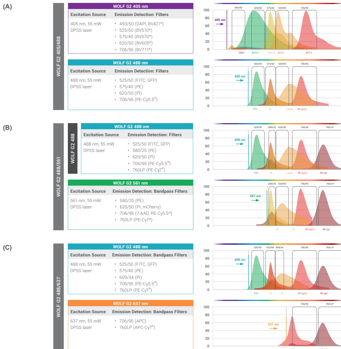
Figure 48. WOLF G2 optical configurations. Each configuration contains a blue (488 nm) laser, plus an additional custom laser (either 405, 561, or 637 nm). This changes the available color number (9 total for 405 and 561 nm configurations, and 7 total for 637 nm configuration). A. 405/488 nm configuration offers 9 fluorescent channels and is best for researchers working with green and blue fluorescent proteins and antibodies. B. 488/561 nm configuration offers 9 fluorescent channels and is best for researchers working with green and red fluorescent proteins and antibodies. C. 488/637 nm configuration offers 7 fluorescent channels and is best for researchers requiring flexibility for work with APC-based antibodies or far-red fluorescent proteins.
