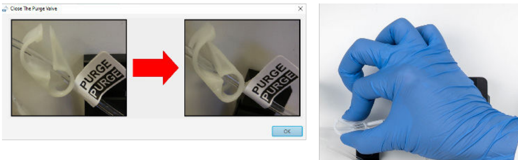
Figure 17. Manually closing the purge valve. See the open (left) and closed (right) valve position. The valve sits above the purge sticker.
