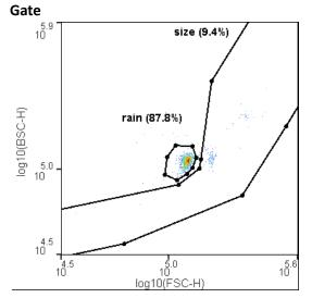
Trigger: FSC Threshold: 8,400 Gain: FL1=FL2=FL3=0.43V, BSC=0.28V
