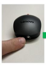
2. Pull on release tab to remove top cover
