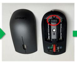
4. Remove the dongle, and insert into PC
