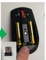
To replace the cover, simply snap the cover back onto the mouse.
