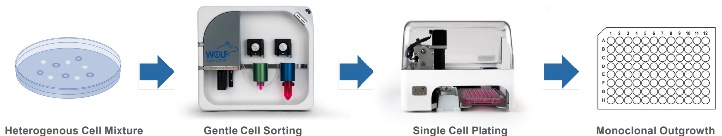
Figure 1. Single-cell cloning workflow: The mixture of cells is collected in a microfuge or FACS tube in buffer of choice and loaded onto the WOLF Cell Sorter with ~50mL of the sheath fluid of choice. Target cells are selected (based on up to 5 optical flow cytometry parameters) and then dispensed into 96-well plates, pre-filled with media. Cells are incubated in culture and imaged or assayed to confirm genetic and monoclonal status.
